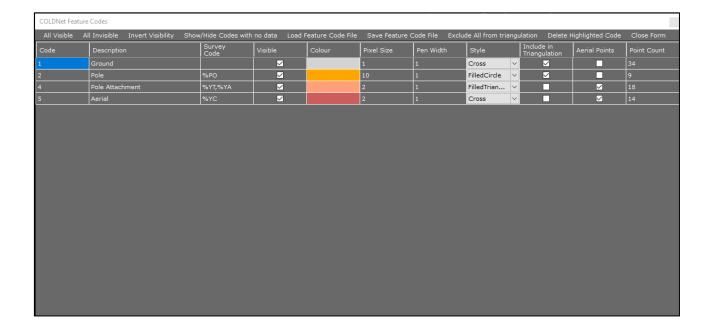
As you can see above, each of the feature codes are split into different data types. These data types are given a default **Description** based on the **Survey Codes** extracted during the import process, however these descriptions and survey codes can be changed if required.
