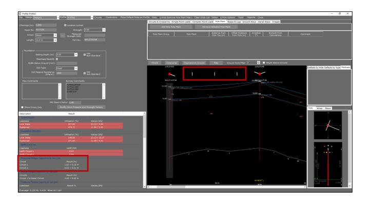
To remove spacers right-click between the span you wish to add them. Select **Spacers** and the circuit and set the number of spacers to zero and select **Save**.
