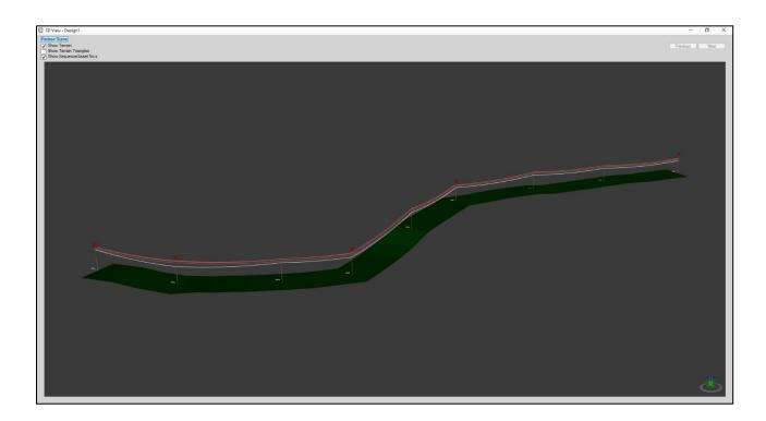
A 3D view of an individual pole and its connecting spans can be achieved by right clicking on the pole of interest in either the main plan view screen or the profile view and selecting **3D View**. A new window will open as shown below when the model is loaded.
